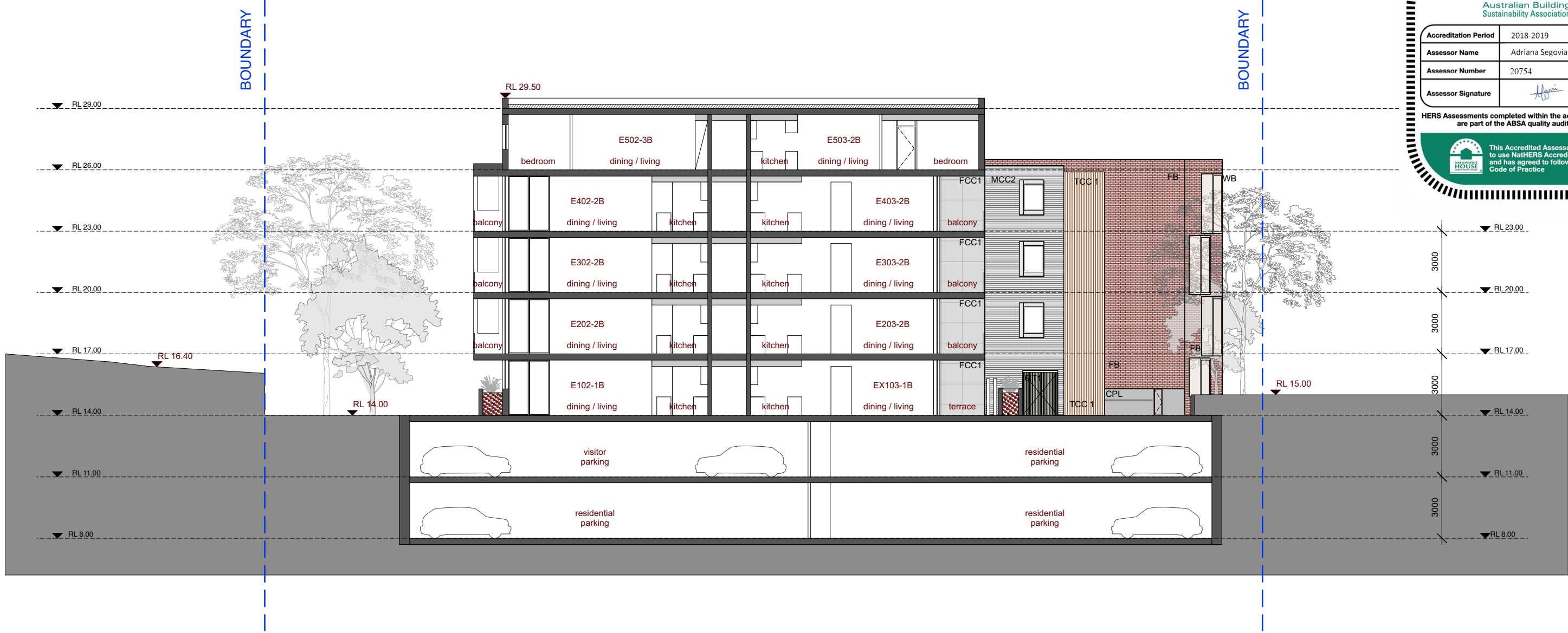
2 A-402 E-W SECTION THROUGH BUILDING E
